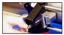
Figure 3-11: Installing the First Transducer
